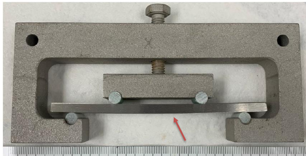
Figure 1-Example of loaded FPB specimen. (excerpt from report)
